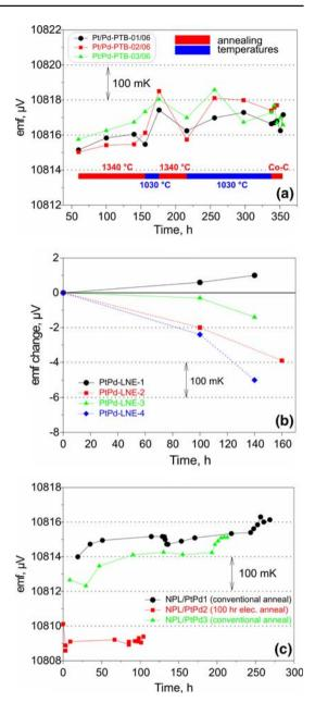
$-2.6\,\mu\text{V}$  (-135 mK) for PtPd-LNE-4 thermocouple (Fig. 1b). The lower stability observed for the PtPd-LNE-2 thermocouple can be explained by the problem encountered during the earliest measurements at the freezing point of silver. The behavior of PtPd-LNE-4 thermocouple is under assessment.
