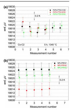
$(\pm 0.1 \text{ K})$  of a single measurement. Therefore, the Pt/Pd-PTB-01/06 and Pt/Pd-PTB-03/06 thermocouples are considered to be thermoelectrically stable, which was also shown by the repeated emf measurements at the freezing point of silver.
